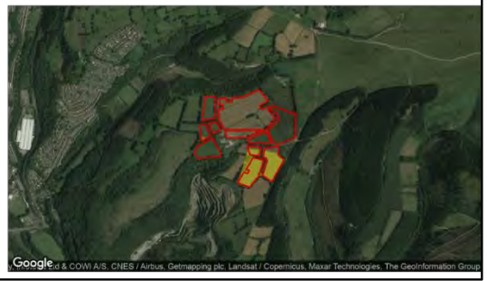
Google Panels: Reflecting (yellow), that would reflect but Sun is behind terrain (orange)
