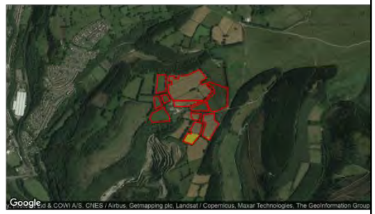
Google Panels: Reflecting (yellow), that would reflect but Sun is behind terrain (orange)
