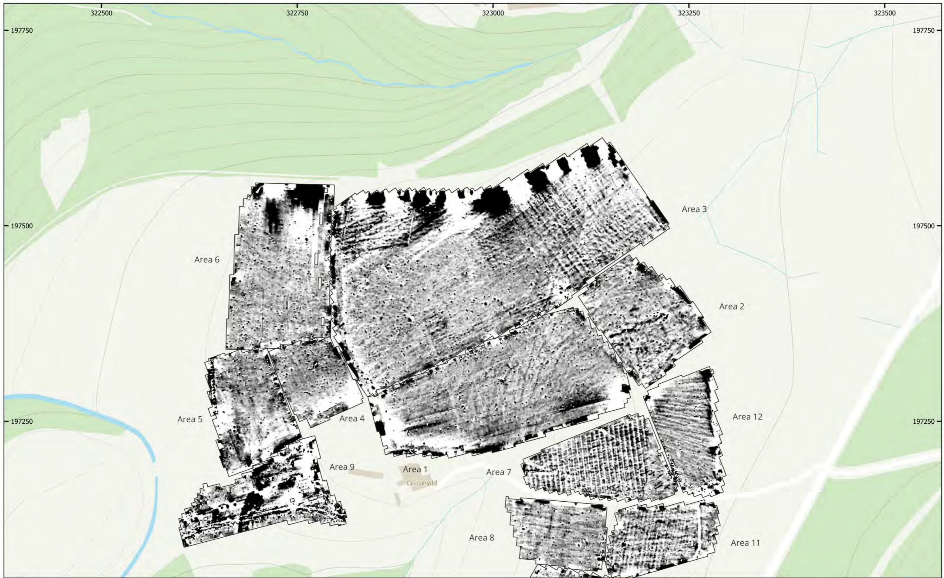
MSST1678: Cyl Lonydd PV Archaeological Survey Figure 3 - Magnetic Total Field (Lower Sensor) (Overview) (North Areas) 1:3,000 @ A3 Copyright Magnitude Surveys Ltd 2024 Contains Ordnance Survey data © Crown Copyright and database right 2024
