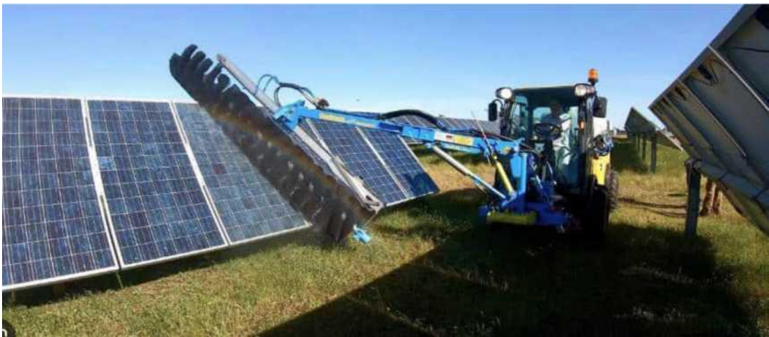
Insert 45: Cleaning of Solar Arrays
